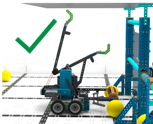
Figure 19: Robots may not vertically expand beyond 19”.
